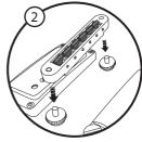
Remove the strings and remove the old bridge by lifting it off the posts. The ResoMax™ comes with posts, but in most instances you can keep using your old posts. Lower your new ResoMax™ bridge onto the posts. Set the intonation "starting point" by adjusting the intonation screws so that the saddles are close to the center of the bridge.
