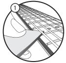
Determine correct string height, by measuring the gap between the top of the 12th fret and the bottom of the low E string. It should be around 0.125" (3mm), or about a stack of 12 business cards if you don't have a ruler. For the high E string, the gap should be around 0.080"(2mm), or about a stack of 8 business cards.
