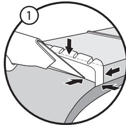
STEP 1. Remove the strings. Trace around the nut (score) every edge of the nut with an exacto knife to prevent lacquer sticking to the nut and the neck and chipping away.
