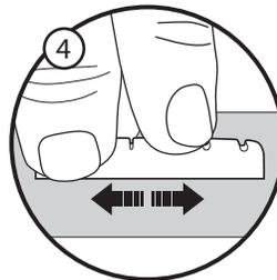
STEP 4. See if your new Graph Tech nut fits into the slot without force. If it's too thick, place a 400 to 600 grit sand paper face up on a flat surface and sand down the sides of the nut until it fits in the slot snugly, but is easily removable.
