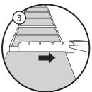
STEP 3. When it is sticking out the side, pull it out in the same direction with a pair of pliers, like you would a tooth. Scrape or file the nut slot free from old glue and finish residue while making sure that the slot remains square.
