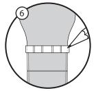
STEP 6. Once you've done the thickness and the height, you just need to sand the ends of the nut so that they are flush with the neck. Just use a pencil and mark the ends of the nut that are sticking out, remove it from the neck and sand it to your marks.
