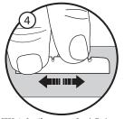
STEP 4. See if your new Graph Tech nut fits into the slot without force. If it's too thick, place a 400 to 600 grit sand paper face up on a flat surface and sand down the sides of the nut until it fits in the slot snugly, but is easily removable.
