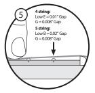
STEP 5. Restring the low E and G strings and tune to pitch to check for correct height. Pushing down on the third note of the low E string should result in a 0.01" gap between the string and the first fret; G string should be 0.008." (5 string bass: low B should have a 0.02" gap and G string should have 0.008")
